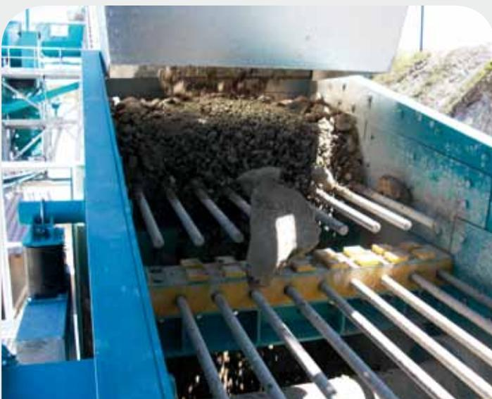
▼ Water-spraying system of a VSK 18/50-2
