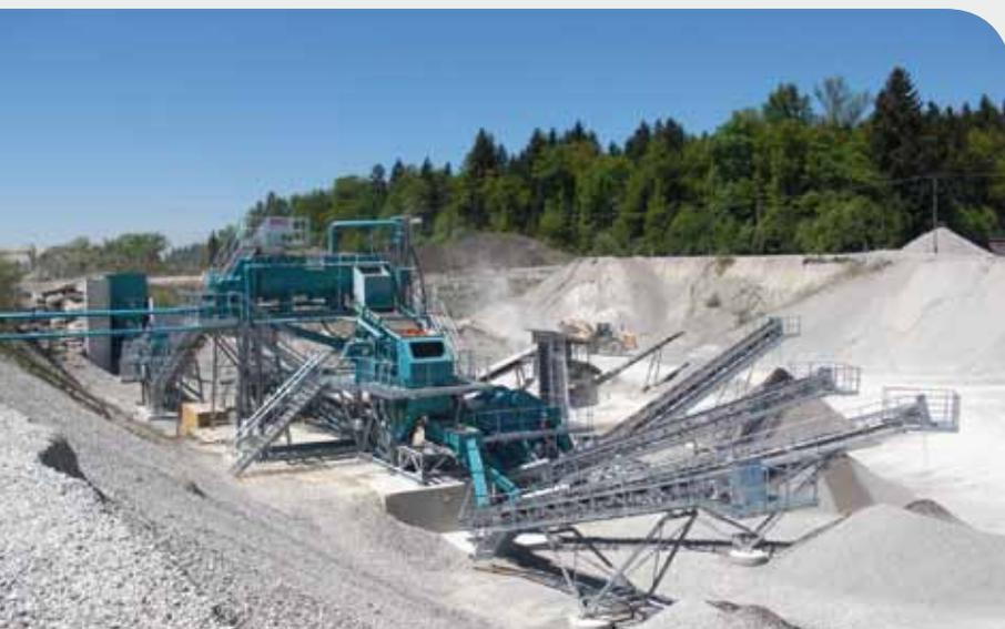
◀ Processing plant near Munich / Germany with pre-crusher, turbowasher, classification and sand processing.
