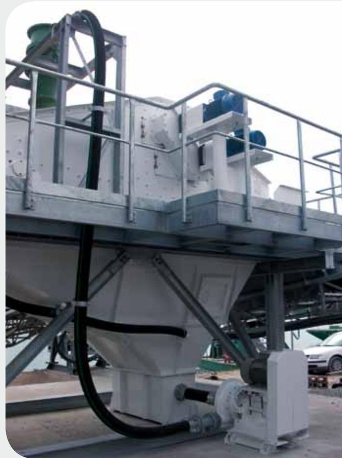
Linear vibrating screening machine VSLW 18/50-1 with pump sump solid matter pump and hydro cyclone classifier for fine sand reclamation ▲
