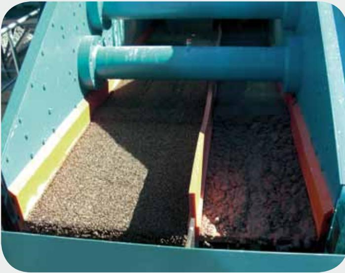
◀ Sand processing with adjustable fine sand removal
